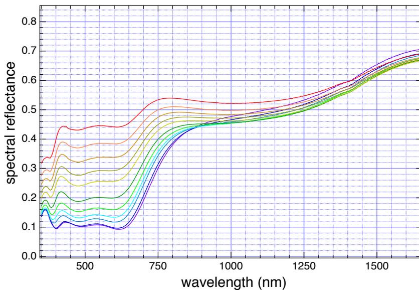
Figure 4: Spectral reflectance of the sun protection insulating glass Pilkington Insulight™ Sun Neutral 68/34. The spectra have been obtained at 11 different angles  $\varphi$  of incidence (in degrees from bottom to top in the range  $350 \text{ nm} < \lambda < 1650 \text{ nm}$ ): 15, 30, 45, 50, 55, 60, 65, 67.5, 70, 72.5, and 75.
