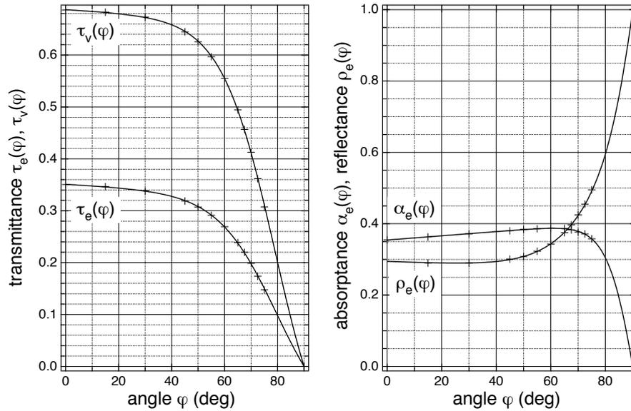
Figure 5:  $\tau_e(\varphi)$ ,  $\tau_v(\varphi)$ ,  $\rho_e(\varphi)$  and  $\alpha_e(\varphi)$  for the insulating glass Pilkington Insulight™ Sun Neutral 68/34. Crosses represent experimental data points whereas the full lines show a fit of a sigmoid function (see text).
