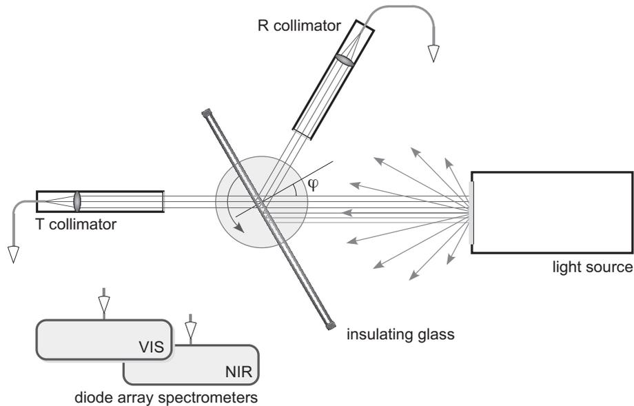
Figure 1: Experimental set-up for spectral optical, angular dependent measurements of both the direct transmittance and reflectance in the near UV, visible and near infrared wavelength range.
