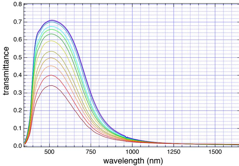
Figure 3: Spectral transmittance of the sun protection insulating glass Pilkington Insulight™ Sun Neutral 68/34. The spectra have been obtained at 12 different angles  $\varphi$  of incidence (in degrees from top to bottom): 0, 15, 30, 45, 50, 55, 60, 65, 67.5, 70, 72.5, and 75.
