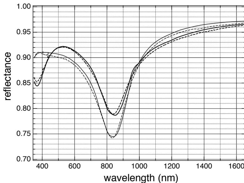
Figure 2: Reflectance of the calibration mirror determined at two angles  $\varphi$  of light incidence,  $15^\circ$  (thicker lines) and  $60^\circ$  (thinner lines). Full and dashed lines represent data obtained via ellipsometric and direct reflectivity measurements, respectively.
