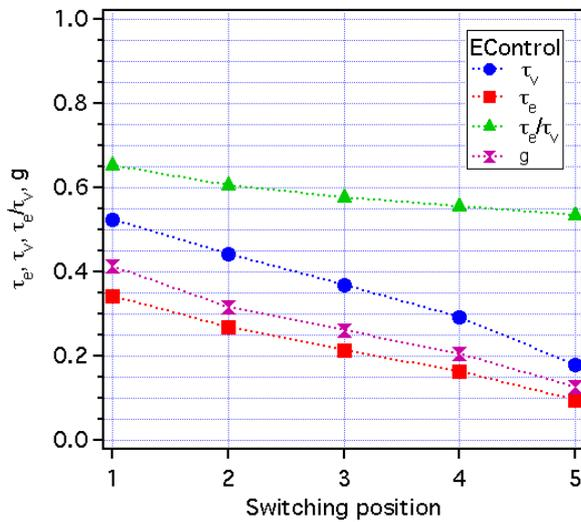
Figure 3: Light transmittance  $\tau_v$ , solar direct transmittance  $\tau_e$ , energy load coefficient  $\tau_e/\tau_v$ , and g-factor for the EControl glass depending on the colouring state. The markers give the values where as the lines are guides for the eyes.
