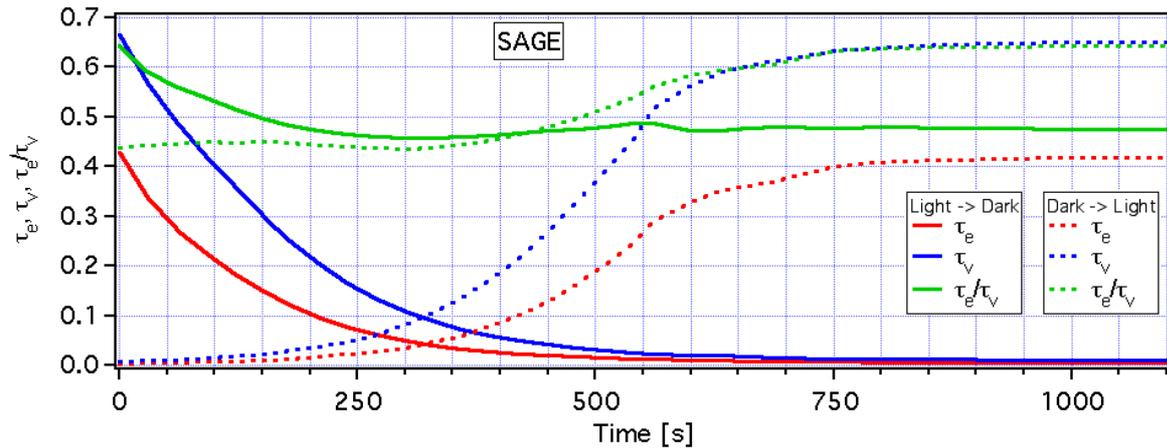
Figure 6: The evolution of the light transmittance  $\tau_v$ , the solar direct transmittance  $\tau_e$ , and the energy load coefficient  $\tau_e/\tau_v$  for the SAGE glass, when switching from bright (1) to dark (2).
