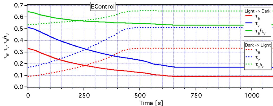
Figure 5: The evolution of the light transmittance  $\tau_v$ , the solar direct transmittance  $\tau_e$ , and the energy load coefficient  $\tau_e/\tau_v$  for the EControl glass, when switching from brightest (1) to darkest (5) transmittance.
