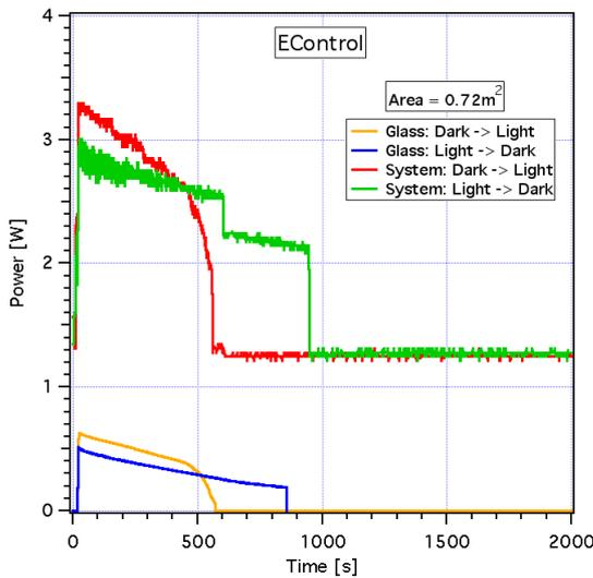
Figure 7: Power consumption of the EControl glass during the switching from the bright (1) state to the darkest (5) state or vice versa and afterwards keeping this status.
